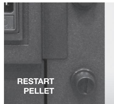
**Pellets temperature safety:** In the rare event there is a too high temperature in the tank, the thermostat for pellets safety with manual reset creates an alarm “ALAR-SIC-FAIL” stopping the pellet boiler stove. You need to reset the system working on the device placed on the back of the stove.
