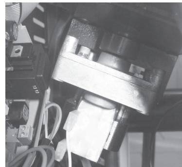
**Reduction motor:** if the motor stops, the stove continues to function until the flame goes out for lack of fuel, and until it has cooled down to the minimum level.
