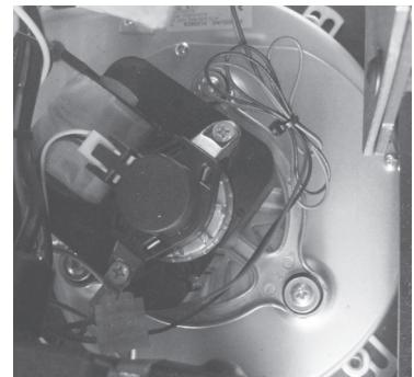
**Flue gas temperature sensor:** thermocouple that measures the temperature of the fumes while keeping the operation or shuts the stove when the flue gas temperature drops below the preset value.
